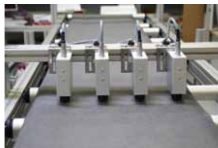
Pic. 14. Prototype EddyCus® Inline for Inline gramature determination by RF EC.
