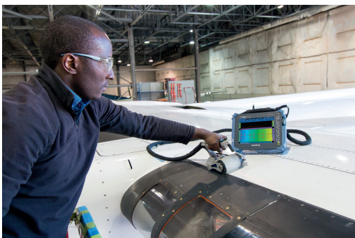
(OmniScan MX2 Phased Array with RollorFORM scanner)
