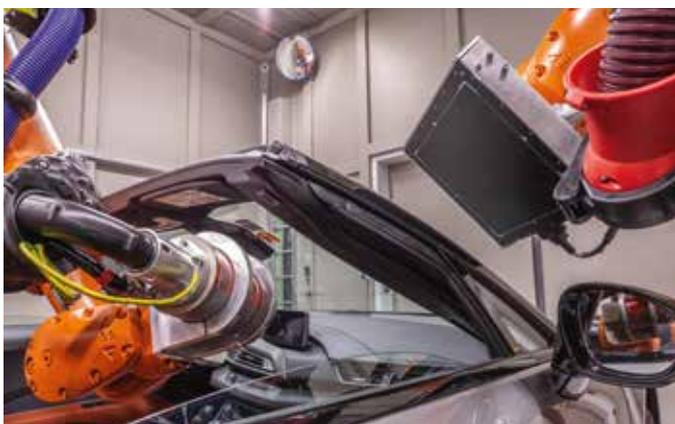
Figure 2 – Robots positioning X-ray source and detector at the A-pillar of a BMW i8 Roadster.
