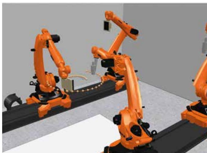
Figure 5 – horizontal acquisition trajectory with a total of 240° scan range around a given ROI.
