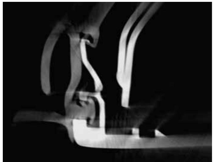
Figure 10 – CT slice orthogonally through the doorframe (on the right), clearly visualizing the door's rubber seal (on the left) and how it snaps into the metal structures.
