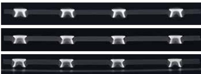
Figure 8 – sagittal CT slice through the row of rivets
