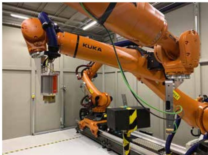
Figure 4 – unobstructed specimen in RoboCT setup with robots at maximum angle of 120°.
