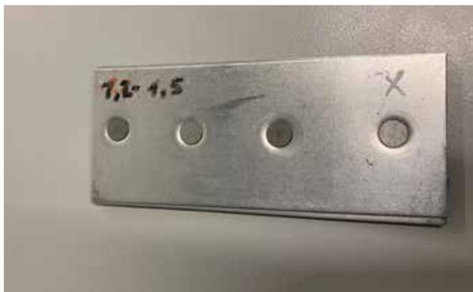
Figure 3 – specimen: rivet joint plates, 110 mm x 50 mm.
